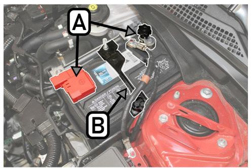
2. Remove the Battery by pulling the Battery Box (A) forward, to give room for it come out, and proceed by pulling the box out as well.
