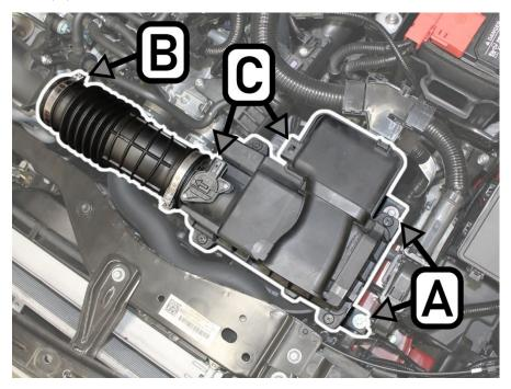
Note: Remove the harness clip to the MAF Sensor by pressing on the two retainer tabs as shown here:
